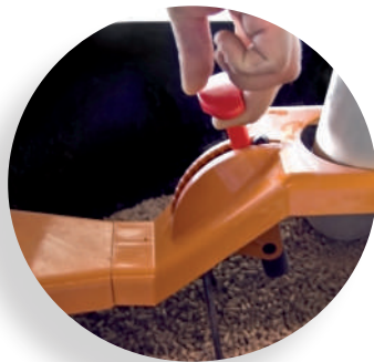
TR2 and TR3D regulation system, for setting when the feeder is full.
